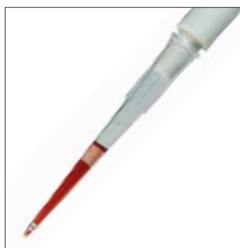
Liquid passes through conventional filter pipet tips causing cross-contamination.
