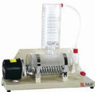
“W4L” Model 4L Basic Water Still, with 304 Stainless-Steel Heater
