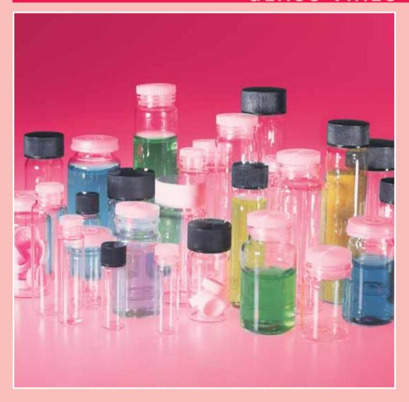
Trident vials are made from neutral glass under the strict conditions required by the pharmaceutical industry. They are available from stock in capacities from 1.75 to 28.25ml, with screw caps, clip-on closures or polythene plugs. Screw neck Trident vials are manufactured with buttress thread, for optimum closure.
