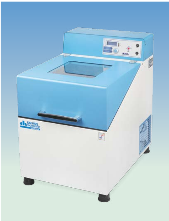
(b) +10°C~+60°C, with Universal Platform “ThermoStable™ IS-20R”
