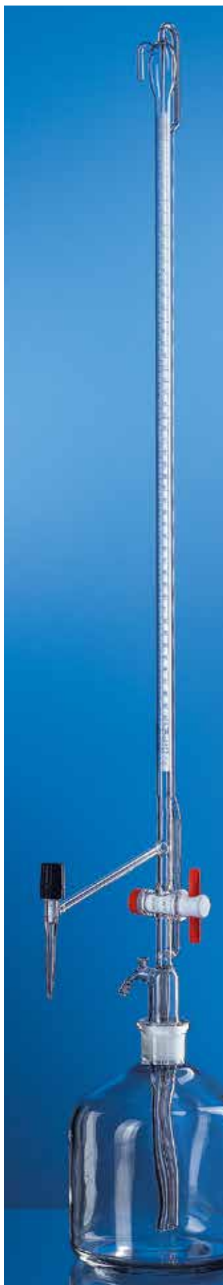
BLAUBRAND® Schellbach Stripe Ring marks at major graduations. Reading at point of contact of the two tips.
