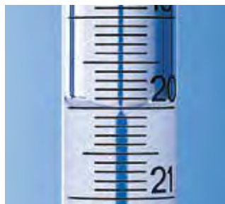
SILBERBRAND Schellbach Stripe Short marks at major graduations. Reading at point of contact of the two tips.
