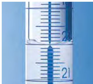
BLAUBRAND® Schellbach Stripe Ring marks at major graduations. Reading at point of contact of the two tips.
