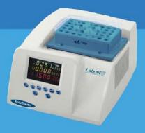
science research applications in the fields of molecular biology, biochemistry and clinical chemistry. It's compact footprint incorporates an intuitive control panel with a large multicolor display, which allows users to easily program and view temperature, time and speed settings. Eight interchangeable aluminum blocks accommodate PCR plates and tubes ranging in size from 0.2mL to 15mL. Designed to meet the of your daily research.
