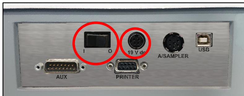
Main switch and 19 VDC power supply socket
