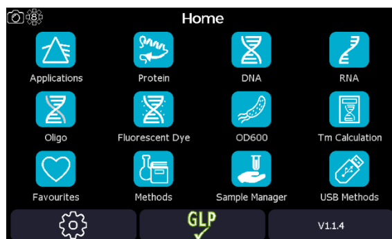
Home screen for the Ultrospec 7500 spectrophotometer displaying the USB memory stick application and screenshot camera icon, made available when a USB flash drive is inserted
